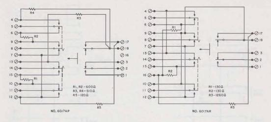
Fig. 3-6017-Type Lever Keys, Schematics (Sheet 4 of 4)
