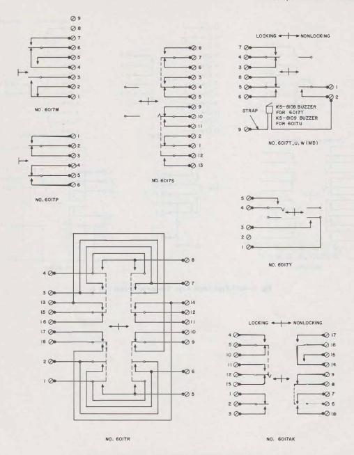
Fig. 3—6017-Type Lever Keys, Schematics (Sheet 2 of 4)
