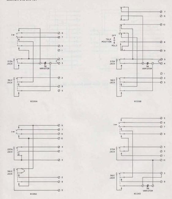
Fig. 4—6026-Type Lever Keys, Schematics
