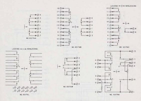
Fig. 3—6017-Type Lever Keys, Schematics (Sheet 3 of 4)
