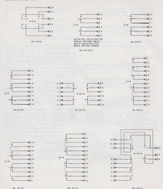
Fig. 3—6017-Type Lever Keys, Schematics (Sheet 1 of 4)
