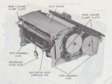
Fig. 8—List 6 Tape Assembly (Rear View)
