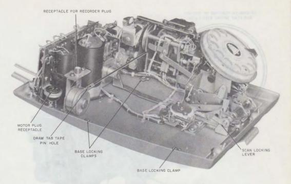
Fig. 10—KS-16844 List 10 Rapidial, With List 12 Tape Assembly Removed
