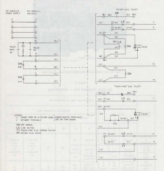
Fig. 13—Typical Connection To Rotary and TOUCH-TONE Dial Equipped Telephone Sets
