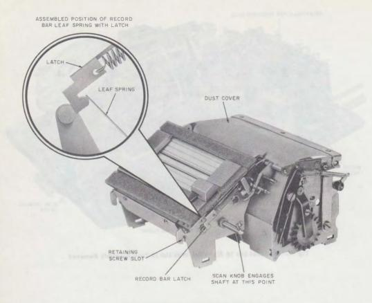
Fig. 11—List 6 Tape Assembly (Front View)
