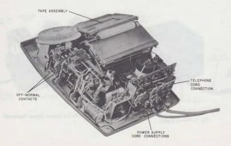
Fig. 5—KS-16844 Rapidial (Housing Removed)
