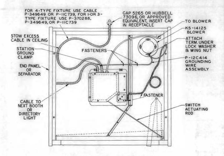
Fig. 4-11-Type Booth Ceiling, Roof Removed
