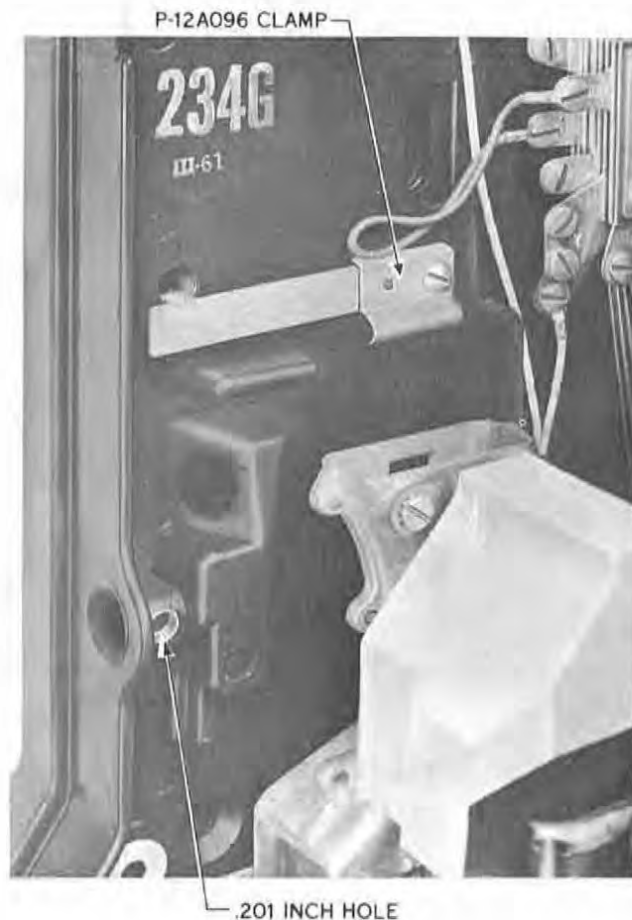
Fig. 6 — Location of Hole for Socket Set Screw
