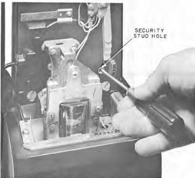
Fig. 25 — Method of Determining if Mounting Surface is Equipped with Four Keyhole Slots
