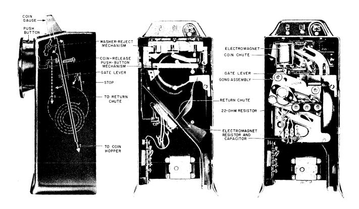
Fig. 2 - Coin-handling Features, Upper Housing
