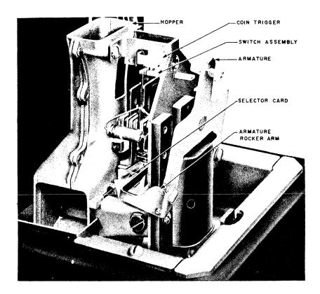
Fig. 8 — Prepay Mechanism Unit, Single-coil, Slow-release Coin Relay
