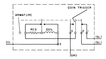
Fig. 10 — P-10E786 Single-coil, Slow-release
