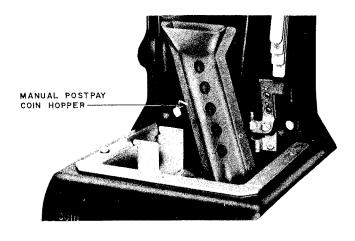
Fig. 5 — Manual Postpay Mechanism Unit
