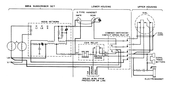
Fig. 1 — Prepay Network-type Coin Collector Circuit
