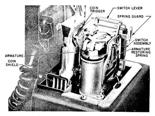
Fig. 6 — Prepay Mechanism Unit, 2-coil Coin Relay
