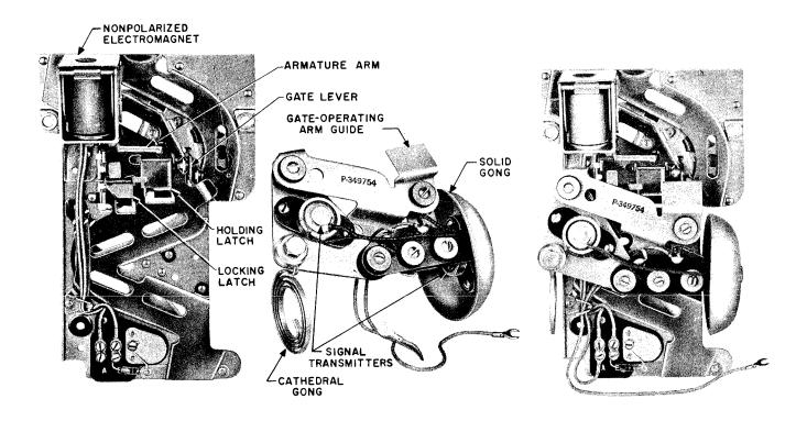
Fig. 3 - Coin Chute and Assembly
