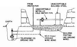
Fig. 8—Acceptable Water System or Building Ground
