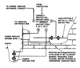
Fig. 5—Acceptable Water System or Building Ground Not Available—MGN Power Service Grounded to Ground Rod
