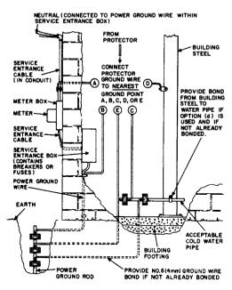
Fig. 4—Acceptable Water System—MGN Power Service
