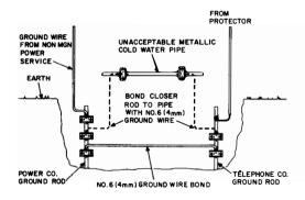
Fig. 6—Acceptable Water System or Building Ground
