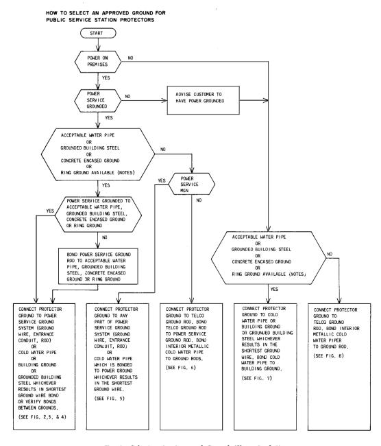
Fig. 1—Selecting An Approved Ground (Sheet 1 of 2)
