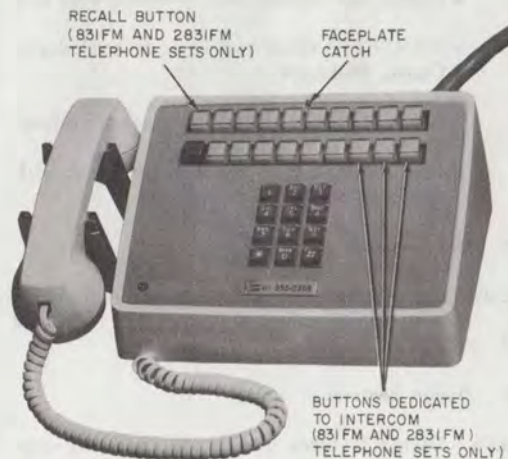
Fig. 1—2831DM (MD) or 2831FM Telephone Set
