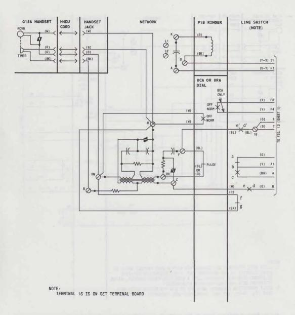
Fig. 8—♦Part of 831CM (Equipped With New Line Switch and Manufactured Before 2-77) Telephone Set,
