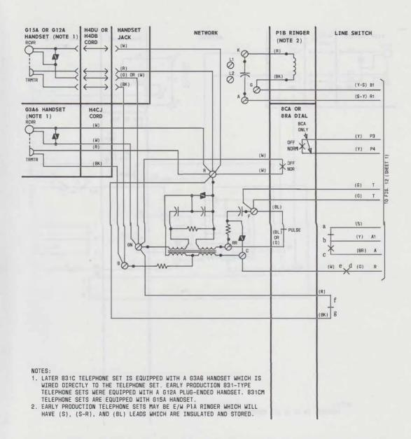
Fig. 7-Part of 831A1M, B1M, C, CT, or CM (Equipped With Old Line Switch) Telephone Set, Connections
