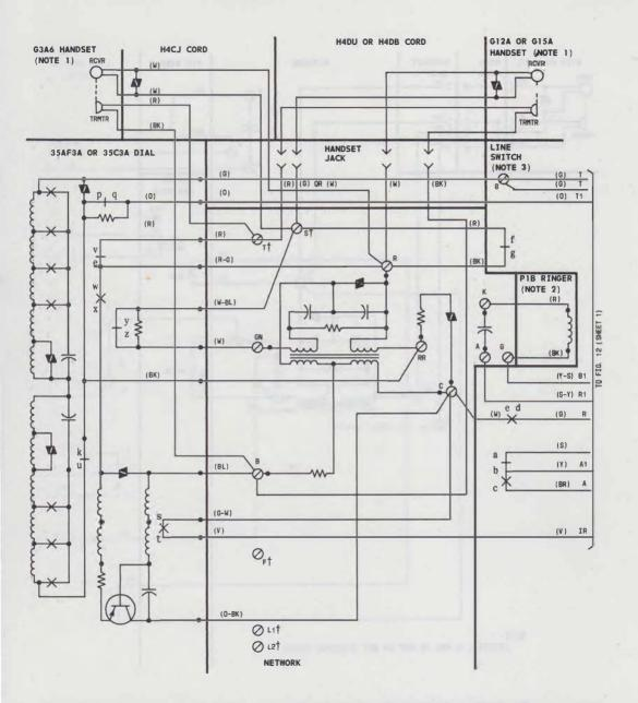
Fig. 10—PPart of 2831A1M, B1M, C, CT, or CM (Equipped With Old Line Switch) Telephone Set, Connections€
