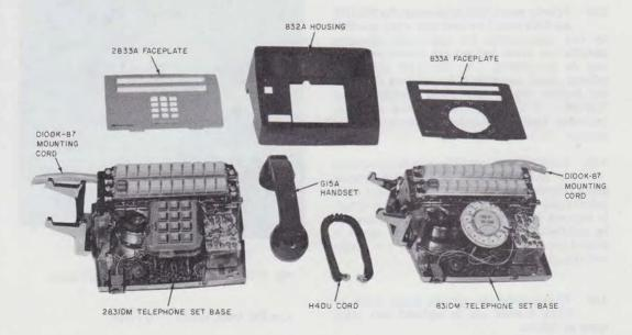
Fig. 2—Station Modular Arrangement, 831DM and 2831DM Telephone Sets
