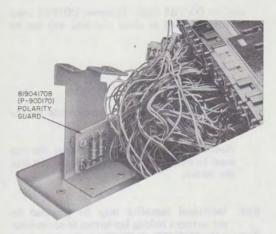
Fig. 4—2831-Type Telephone Set with 819041708 (P-90D170) Polarity Guard Installed
