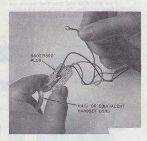
Fig. 5—Installing Spade-Tipped Handset Cords
