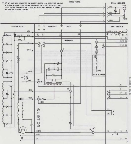
Fig. 11—PPart of 2831CM (Equipped With New Line Switch) Telephone Set, Connections
