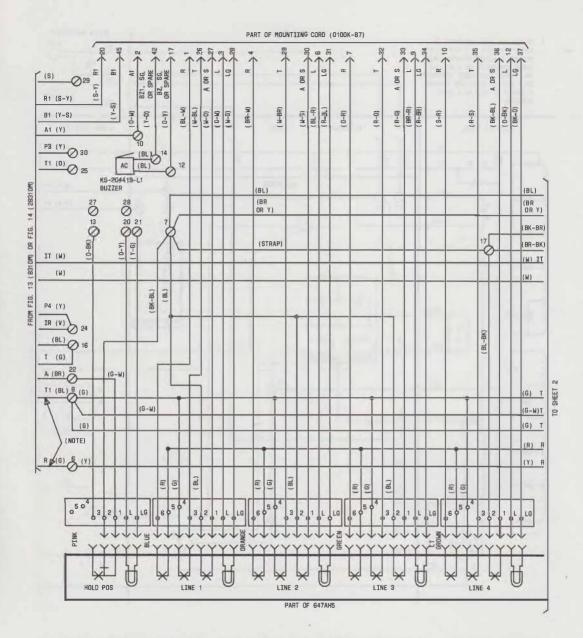
Fig. 15—₱831DM or 2831DM Telephone Set, Key and Mounting Cord Arrangement (Sheet 1 of 4)●
