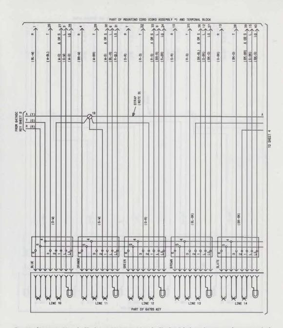
Fig. 12—♥831A1M, B1M, C, CT, CM or 2831A1M, B1M, C, CT, CM Telephone Set, Key and Mounting Cord Arrangement (Sheet 3 of 4)€
