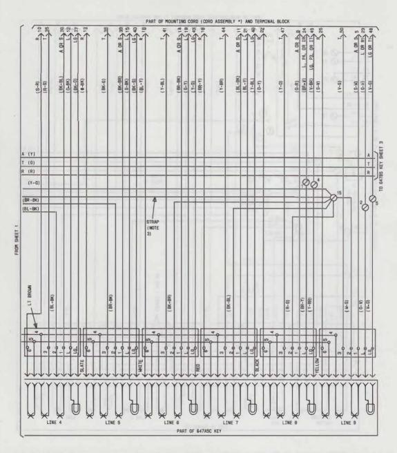
Fig. 12—♦831A1M, B1M, C, CT, CM or 2831A1M, B1M, C, CT, CM Telephone Set, Key and Mounting Cord Arrangement (Sheet 2 of 4)♦
