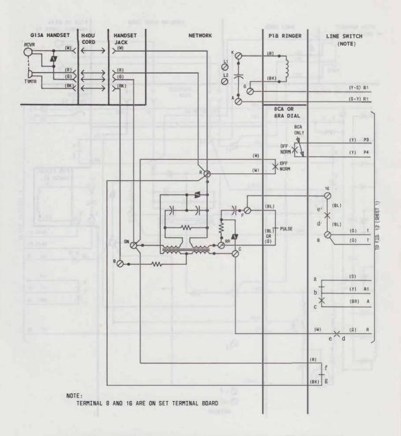
Fig. 9—Part of 831CM (Manufactured 2-77 or later) Telephone Set, Connections
