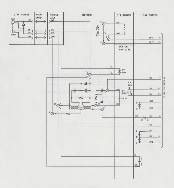
Fig. 13—Part of 831DM Telephone Set, Connections
