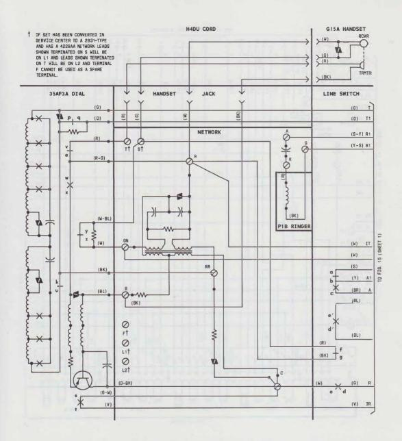
Fig. 14—Part of 2831DM Telephone Set, Connections
