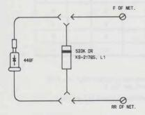
Fig. 6—Installing Diode for Dial Restriction
