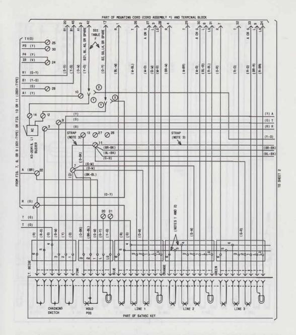
Fig. 12—₱831A1M, B1M, C, CT, CM or 2831A1M, B1M, C, CT, CM Telephone Set, Key and Mounting Cord Arrangement (Sheet 1 of 4)◀
