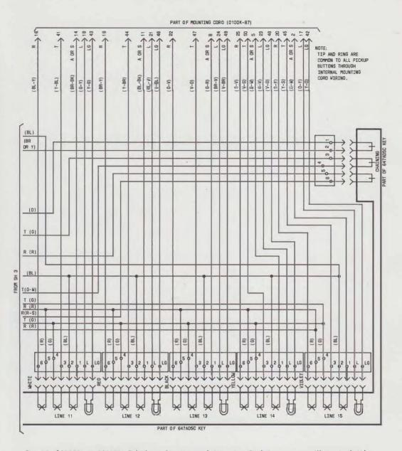
Fig. 15—₱831DM or 2831DM Telephone Set, Key and Mounting Cord Arrangement (Sheet 4 of 4)€
