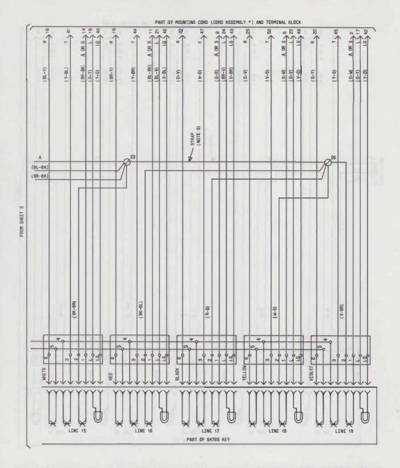
Fig. 12—₱831A1M, B1M, C, CT, CM or 2831A1M, B1M, C, CT, CM Telephone Set, Key and Mounting Cord Arrangement (Sheet 4 of 4) ♦
