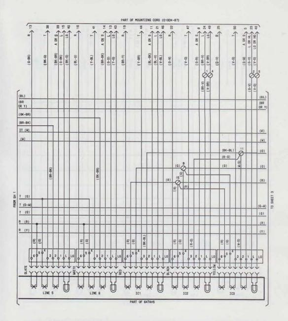
Fig. 15—₱831DM or 2831DM Telephone Set, Key and Mounting Cord Arrangement (Sheet 2 of 4)€
