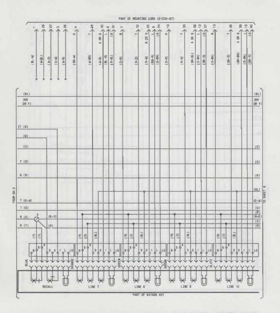
Fig. 15-\$31DM or 2831DM Telephone Set, Key and Mounting Cord Arrangement (Sheet 3 of 4)
