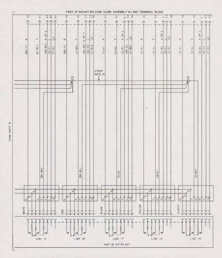
Fig. 9-\$831- and 2831-Type Telephone Set, Connections (Sheet 6 of 6)
