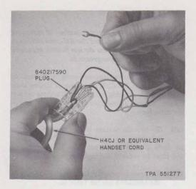
Fig. 5—Installing Spade-Tipped Handset Cords
