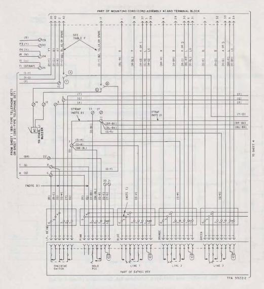
Fig. 9-\$31- and 2831-Type Telephone Set, Connections (Sheet 3 of 6)
