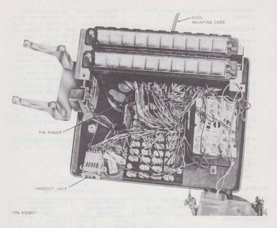
Fig. 4—2831CT (MD) Telephone Set, Dial Removed
