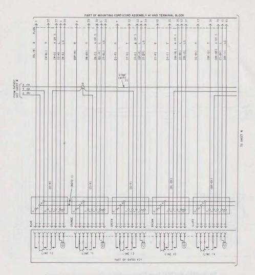
Fig. 9-\$31- and 2831-Type Telephone Set, Connections (Sheet 5 of 6)
