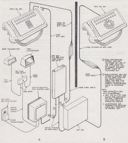
A-INSTALLATION OF TELEPHONE SET AND 3-TYPE SPEAKERPHONE COMPONENTS 8-TELEPHONE SET INSTALLATION (WITHOUT 3-TYPE SPEAKERPHONE)
