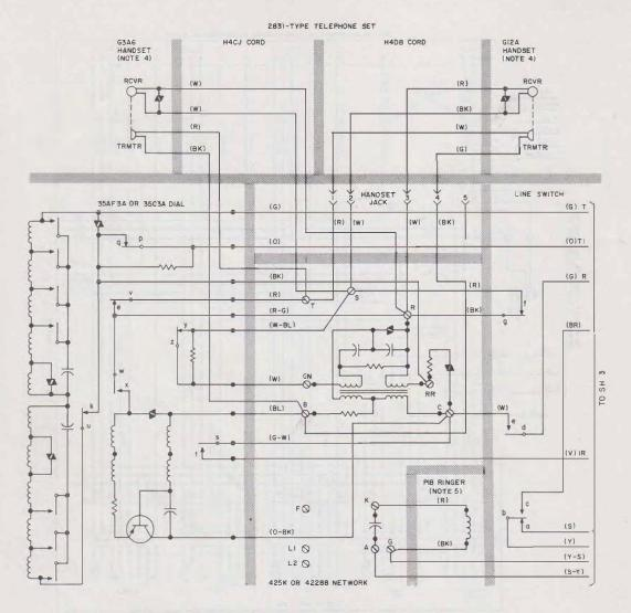
Fig. 9-\$31- and 2831-Type Telephone Set, Connections (Sheet 2 of 6)
