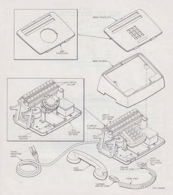
Fig. 6-\$Station Modular Arrangement, 831- and 2831-Type Telephone Sets
