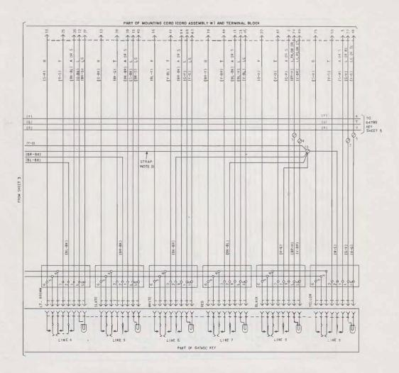
Fig. 9-\$31- and 2831-Type Telephone Set, Connections (Sheet 4 of 6)
