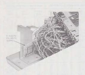
Fig. 8—2831-Type Telephone Set with P-90D170 **Polarity Guard Installed**
