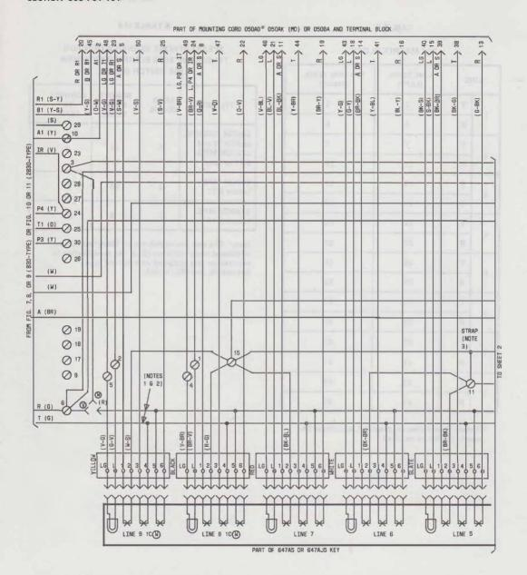
Fig. 12—₱830- or 2830-Type Telephone Set, Key and Mounting Cord Arrangement (Sheet 1 of 2)₱
