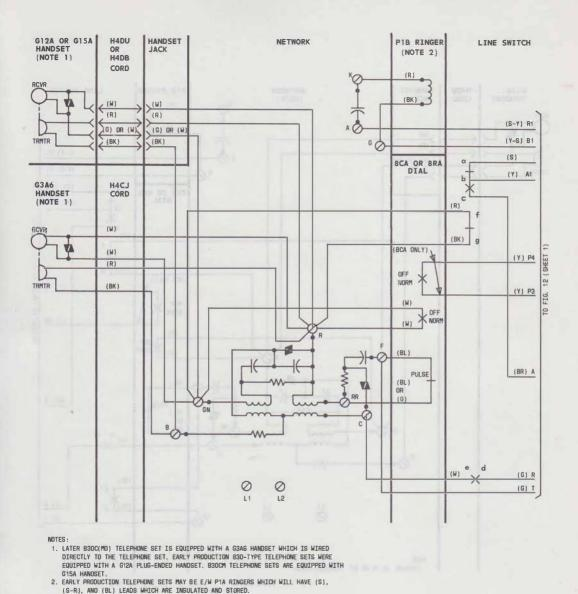
Fig. 7-PPart of 830A1M, B1M, C, CT, or CM (Equipped With Old Line Switch) Telephone Set, Connections♥
