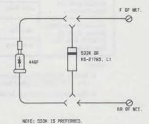
Fig. 6—Installing Diode for Dial Restriction
