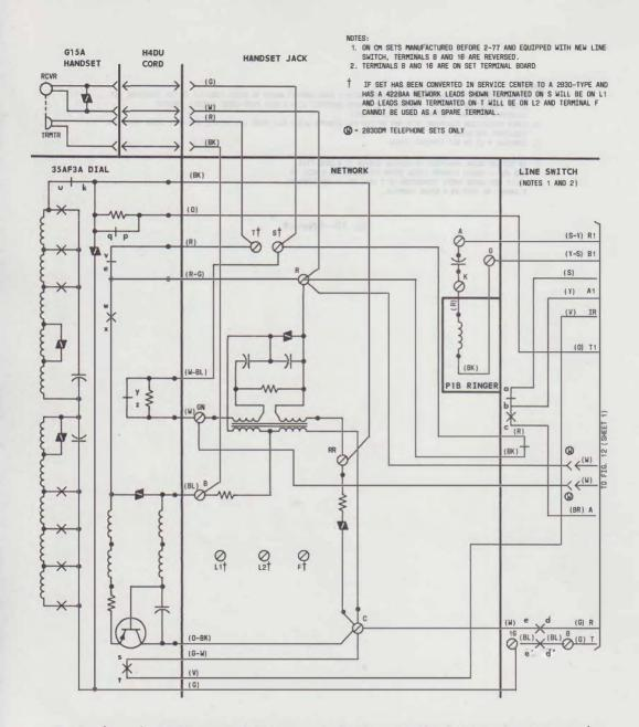
Fig. 11—PPart of 2830CM (Equipped With New Line Switch) or 2830DM Telephone Set, Connections
