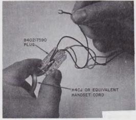
Fig. 5—Installation of Spade-Tipped Handset Cords
