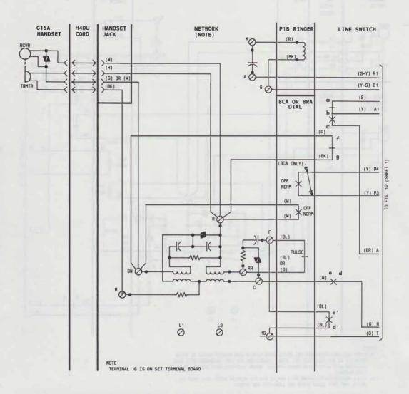
Fig. 8—₱Part of 830CM (Equipped With New Line Switch and Manufactured Before 2-77) Telephone Set,
