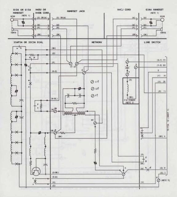
Fig. 10-Part of 2830A1M, B1M, C, CT, or CM (Equipped With Old Line Switch) Telephone Set, Connections
