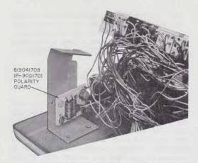
Fig. 4—819041708 (P-90D170) Polarity Guard, Installed
