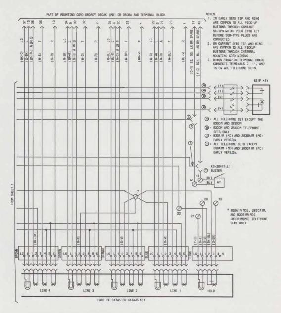
Fig. 12—₱830- or 2830-Type Telephone Set, Key and Mounting Cord Arrangement (Sheet 2 of 2)€
