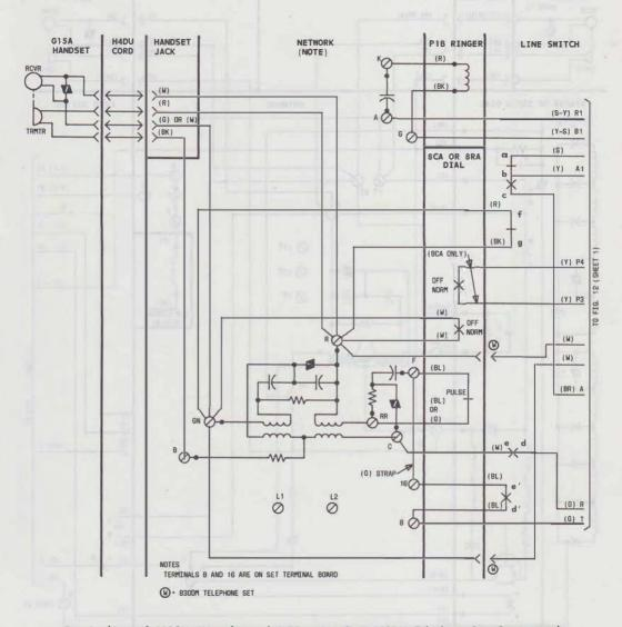
Fig. 9—Part of 830CM (Manufactured 2-77 or Later) or 830DM Telephone Set, Connections
