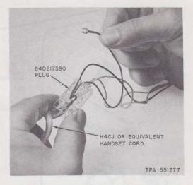
Fig. 7—Installation Spade-Tipped Handset Cords
