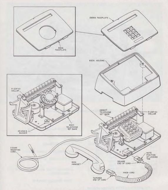
Fig. 5-\$Station Modular Arrangement, 830- and 2830-Type Telephone Sets#
