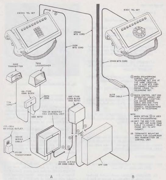
A - INSTALLATION OF TELEPHONE SET AND 3-TYPE SPEAKERPHONE COMPONENTS B-TELEPHONE SET INSTALLATION (WITHOUT 3-TYPE SPEAKERPHONE)
