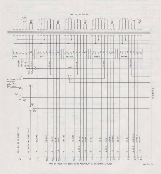
Fig. 9—830- and 2830-Type Telephone Set Connections (Sheet 1 of 4)
