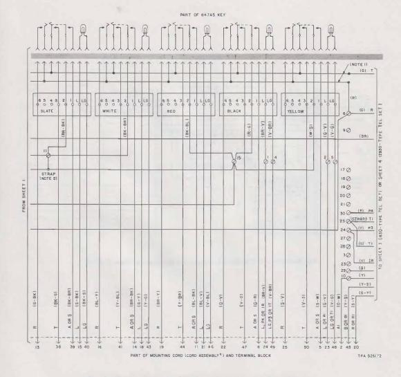
Fig. 9—830- and 2830-Type Telephone Set Connections (Sheet 2 of 4)
