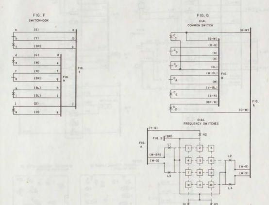
Fig. 8-2872A1M or 2872A2M Telephone Set, Connections (Sheet 3 of 5)
