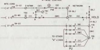
Fig. 12-2872A1M or 2871A2M Telephone Set-2/4-Wire Connections
