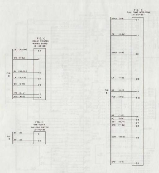
Fig. 8-2872A1M or 2872A2M Telephone Set, Connections (Sheet 2 of 5)
