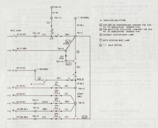
Fig. 9—"I" Hold, Exclusion, Station Busy Lamp, and Add-On Conferencing—1A1 and 1A2 KTS (Showing 5th Key Modified)
