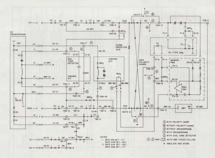
Fig. 14—2872A1M or 2872A2M Telephone Set, Partial Functional Schematic
