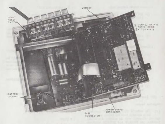
Fig. 5-2872A2M Telephone Set, Internal View, Overall
