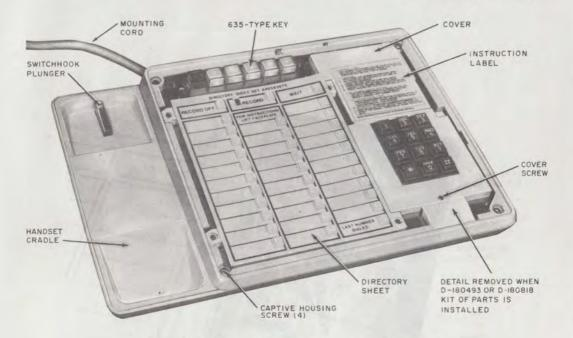
Fig. 2—2872A2M Telephone Set—Faceplate and Handset Removed
