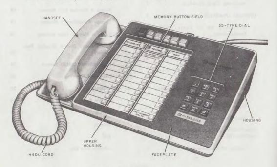
Fig. 1-2872A1M (MD) or 282A2M Telephone Set
