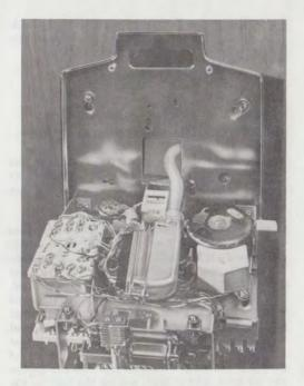
Fig. 9—Connector Cable and D-180375 Kit of Parts (Early Version)
