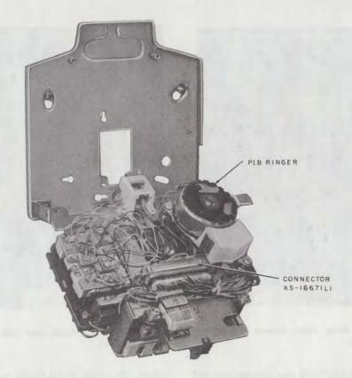
Fig. 6-851CM or 2851CM Telephone Set Showing KS-16671L1 Mounting Cord Connector
