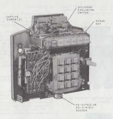
Fig. 5-2851CM Telephone Set With Exclusion (Housing Removed)
