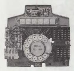
rig. 3—Early Version 851-Type Telephone Set Base (Housing Removed)
