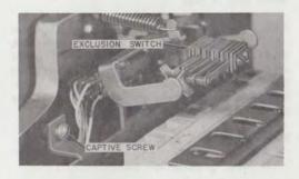
Fig. 10—Exlusion Switch Installed and Hinged Chassis Mounting Screws (Early Version)
