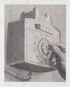
Fig. 15—Installing 851A(MD) or 852A Faceplate
