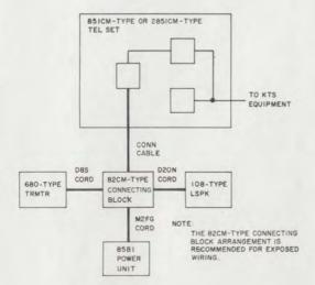
Fig. 22-Block Diagram of 4A Speakerphone Located at Station Using 82-Type Adapter
