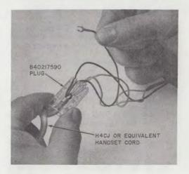
Fig. 14—Installing Spade-Tipped Handset Cords in Early Production 851- and 2851-Type Telephone Sets with G12A Handset
