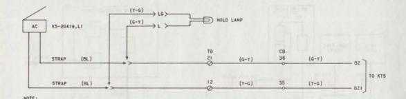
Fig. 25—Hold Lamp Connections
