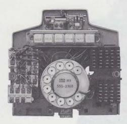
Fig. 3—Early Version 851-Type Telephone Set Base (Housing Removed)
