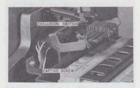
Fig. 10—Exclusion Switch Installed and Hinged Chassis Mounting Screws (Early Version)
