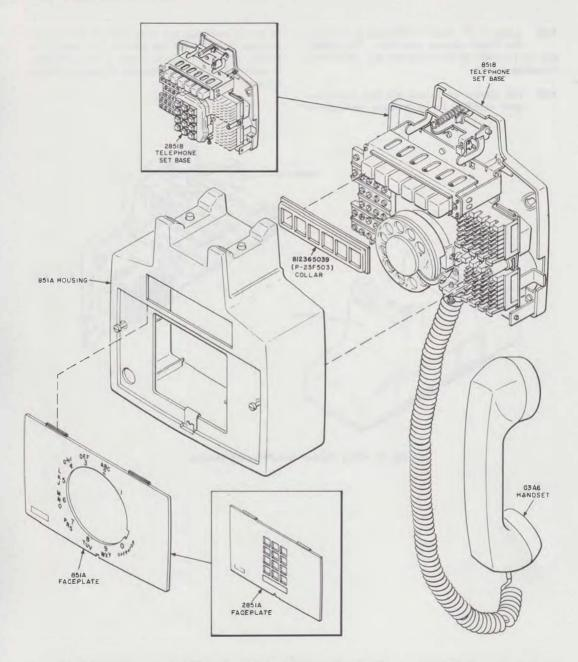
Fig. 18—Station Arrangement, 851BT and 2851BT Telephone Set Showing Current 851A Housing and Base Plate
