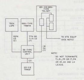
Fig. 21—Block Diagram, Control Unit Located Near Station
