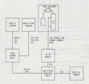
Fig. 22-Block Diagram, Control Unit Located at KTS Equipment
