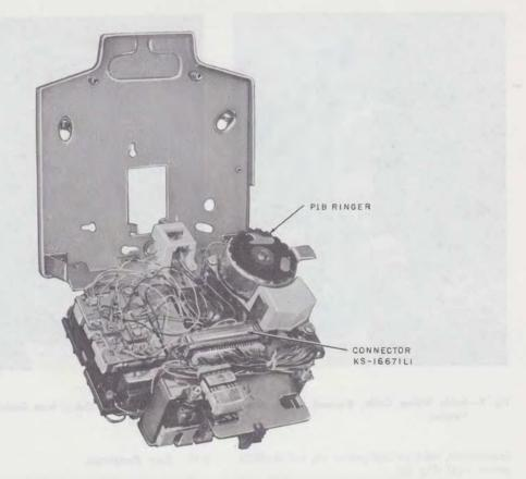
Fig. 6-851CM or 2851CM Telephone Set Showing KS-16671L1 Mounting Cord Connector
