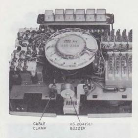
Fig. 13—KS-20419L1 Buzzer Mounted on 851-Type Telephone Set
