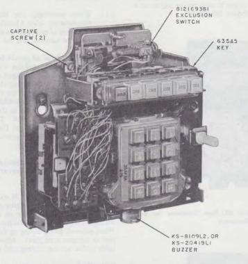
Fig. 5—2851CM Telephone Set (Housing Removed)
