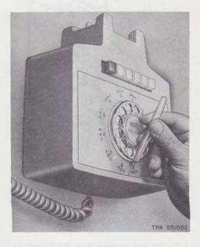
Fig. 15—Installing 851A(MD) or 852A Faceplate
