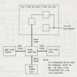
Fig. 23—Block Diagram of 4A Speakerphone Located at Station
