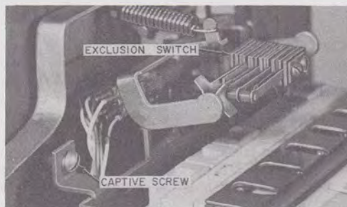
Fig. 13—Exclusion Switch Installed and Hinged Chassis Mounting Screws
