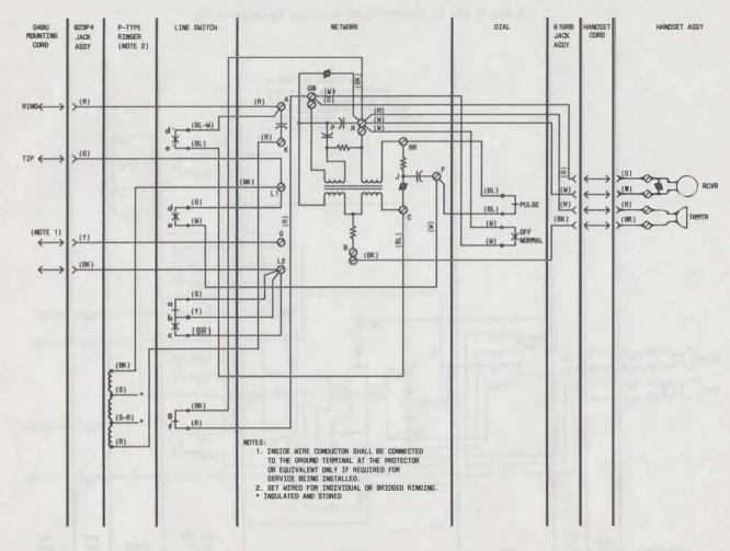
Fig. 4-951A 1-03 Telephone Set, Connections
