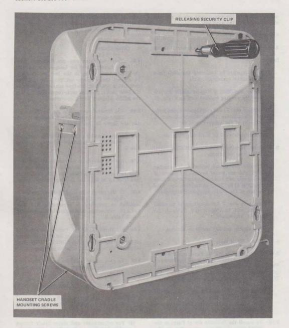
Fig. 5—950A- or 2950A-Type Telephone Set With Panel and Frame Removed
