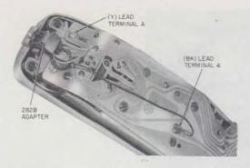
Fig. 6—282A (MD) or 282B Adapter (P/O D-180825 Kit of Parts) Installed in Hand Telephone Set
