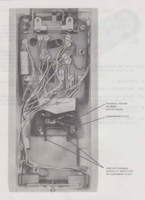
Fig. 7—Terminal Board (P/O D-180825 Kit of Parts) Installed in Housing
