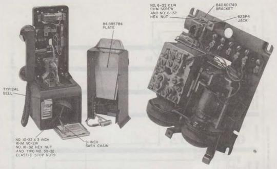
Fig. 5—Decorator Set Showing D-180573 Kit of Parts Installed
