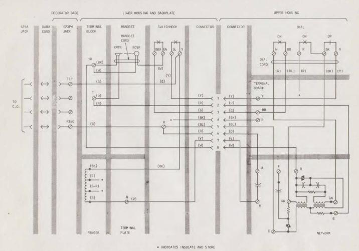
Fig. 11—♦Connections for D-180574 Coin Decorator Telephone Set, Wall Mounted Without a Subset♦
