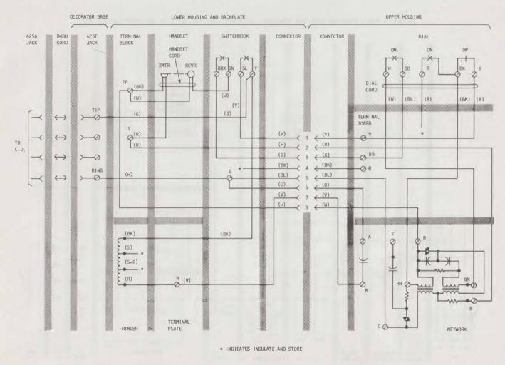
Fig. 9—♦Connections for D-180574 Coin Decorator Telephone Set Using a Decorator Base Without Subset
