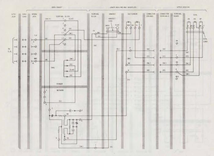
Fig. 10—♦Connections for D-180574 Coin Decorator Telephone Set, Wall Mounted Using a Subset♦
