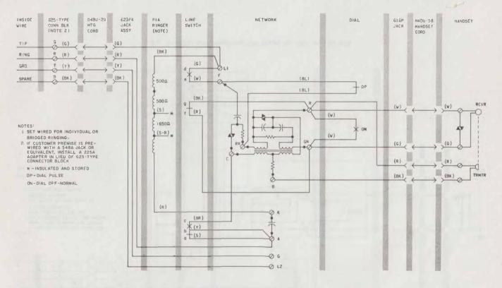
Fig. 2-882A200 Telephone Set, Connections
