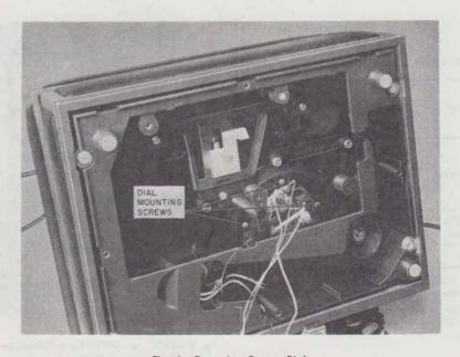
Fig. 6—Removing Rotary Dial
