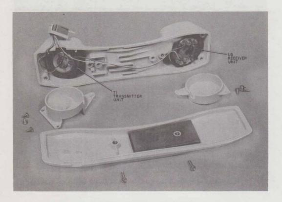
Fig. 11—Removing Transmitter and Receiver Units From Handset (A Code Sets Only)
