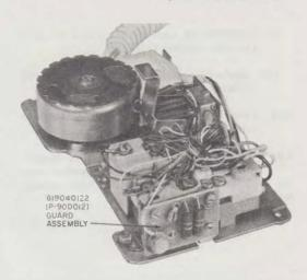
Fig. 3—819040122 (P-90D012) Guard Assembly (Polarity Guard) Installed on Telephone Set
