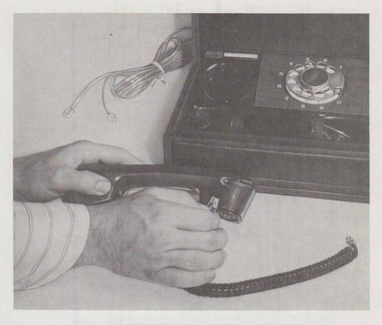
Fig. 12—881C100 Telephone Set—Removing Handset Cord From Handset
