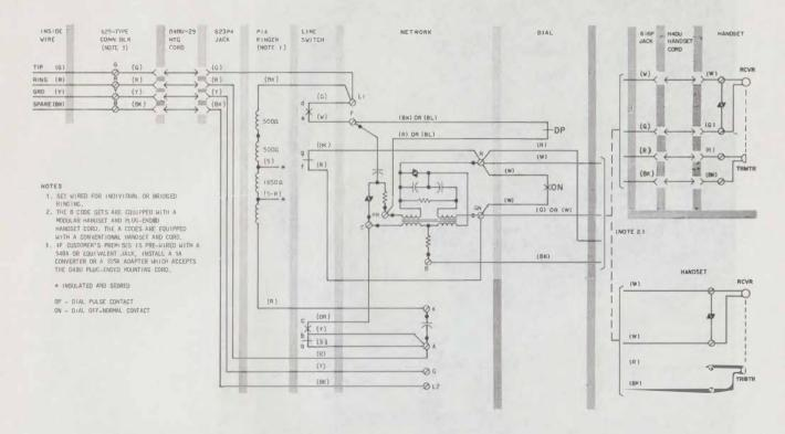
Fig. 13—₱881A100 (MD), 881B100 (MD), 881A101 (MD), 881B101 (MD), or 881B110 (MD) Telephone Set, Connections ●
