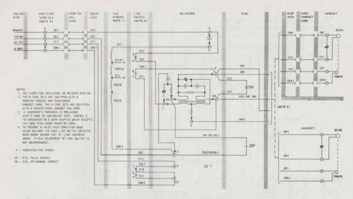
Fig. 15—₱881A100 (MD), 881B100 (MD), 881A101 (MD), 881B101 (MD), or 881B110 (MD) Telephone Set Wired for 1A1 or 1A2 KTS€
