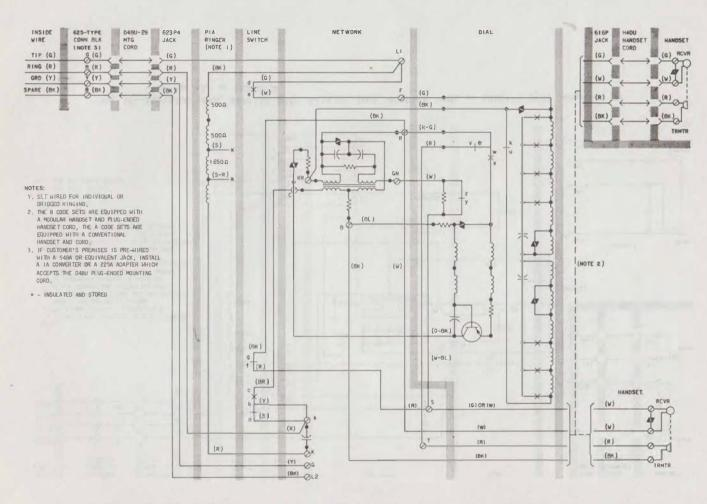
Fig. 14-#2881A100 (MD), 2881A101 (MD), 2881B100 (MD) 2881B101 (MD), or 2881B110 (MD) Telephone Set, Connections
