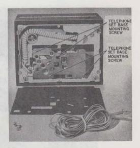
Fig. 5—881C- or 2881C-Type Telephone Set With Bottom Cover Removed
