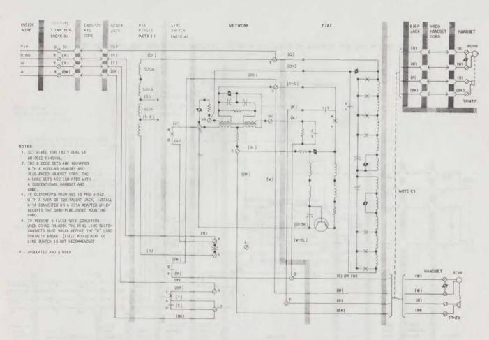
Fig. 16—02881A100 (MD), 2881B100 (MD), 2881A101 (MD), 2881B101 (MD), or 2881B110 (MD) Telephone Set Wires for 1A1 or 1A2 KTS0
