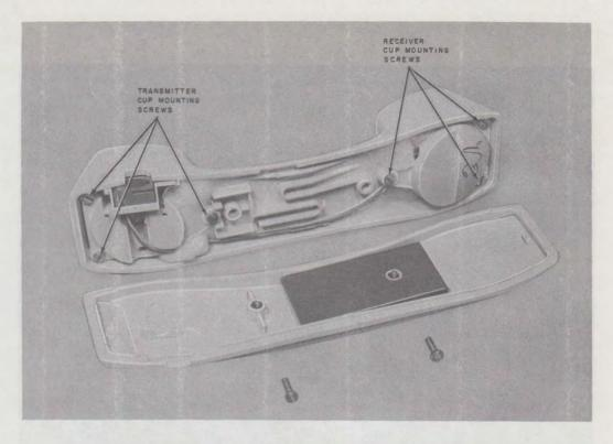
Fig. 10—Removing Transmitter and Receiver Cups From Handset (A Code Sets Only)
