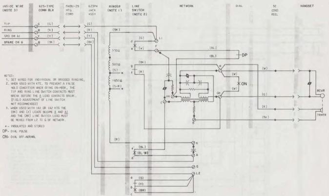
Fig. 2-911A1-03 Telephone Set, Connections
