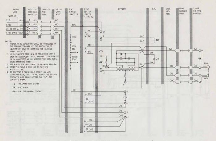
Fig. 4—\$940D40-62 and 940D41-50 Telephone Set, Connections\$
