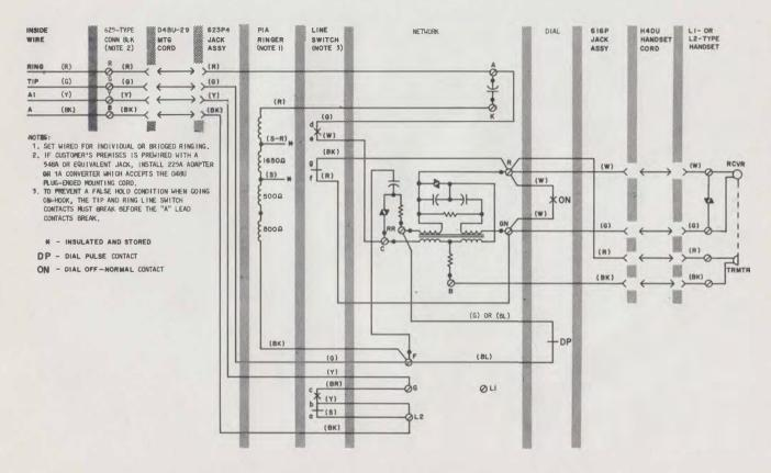
Fig. 5-940A (MD), 940B (MD), and 940C (MD) Telephone Set Connections, Wired for 1A1 or 1A2 KTS
