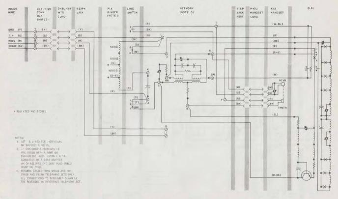
Fig. 9-2930A-(MD), 2930B-, or 2931B-Type Telephone Set, Connections
