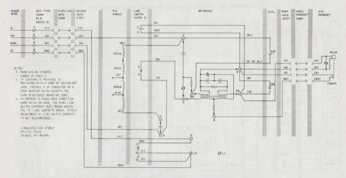
Fig. 10-930A-(MD) or 930B-Type Telephone Set Wired for 1A1 or 1A2 KTS
