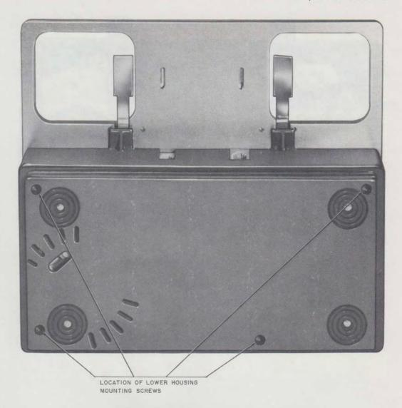
Fig. 6-930B-, 2930B-, or 2931B-Type Telephone Set, Bottom View
