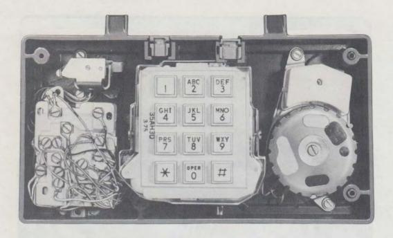
Fig. 7—2930B-Type Telephone Set, Upper Housing, and Handset Mounting Plate Removed
