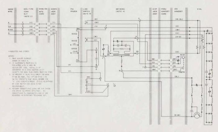
Fig. 11—2930A-(MD), 2930B-, or 2931B-Type Telephone Set Wired for 1A1 or 1A2 KTS
