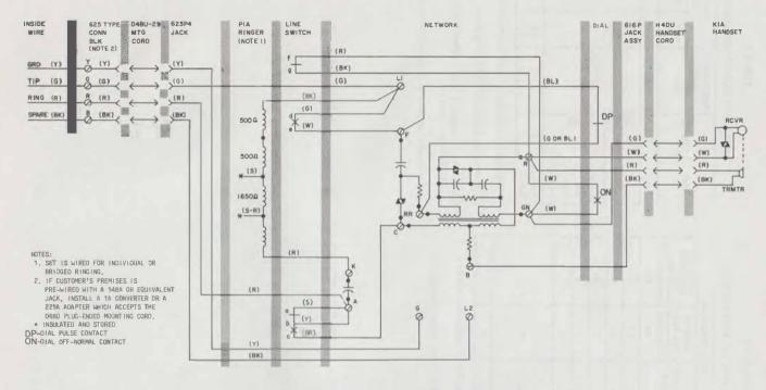
Fig. 8-930A-(MD) or 930B-Type Telephone Set, Connections
