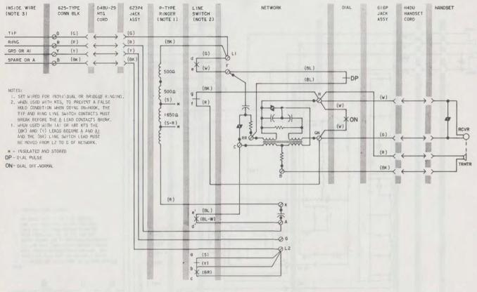
Fig. 3-902A1 Telephone Set, Connections
