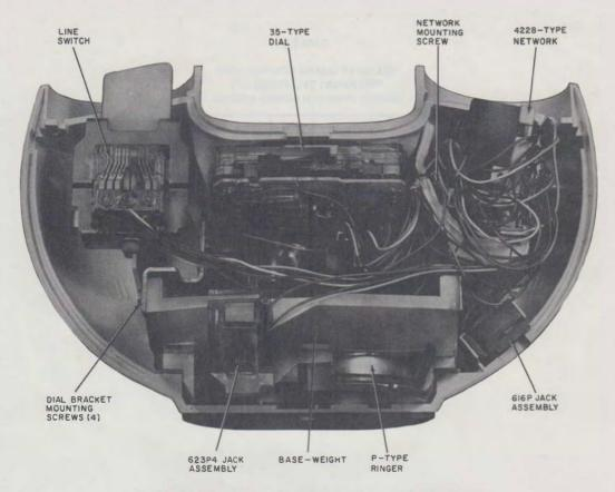
Fig. 2—2902A1 Telephone Set With Two-Piece Housing Separated
