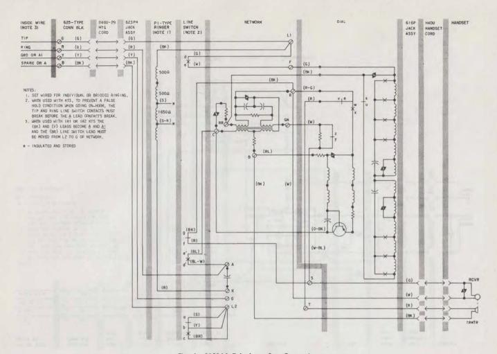
Fig. 4-2902A1 Telephone Set, Connections
