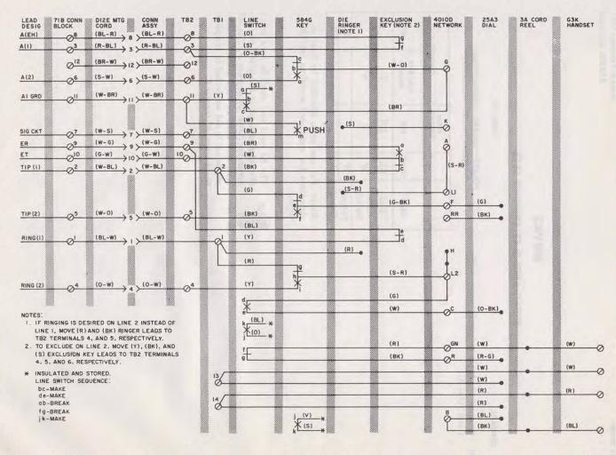
▶Fig. 2—1751C and D Telephone Set Connections With 25A3 (MD) Dial
