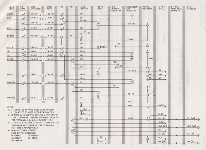
♦Fig. 1—1751C and D Telephone Set Connections With 25W3 (MD) Dial
