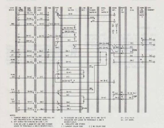
Fig. 1—\$751A (MD) and 751B (MD) Telephone Sets, Connections\$
