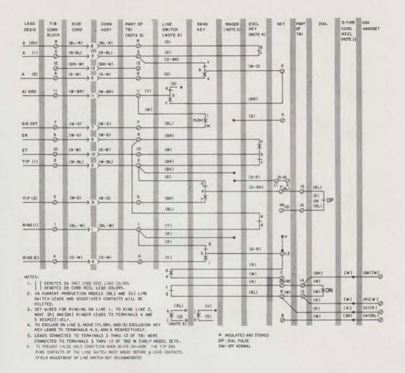
Fig. 2-\$751C and 751D Telephone Sets, Connections
