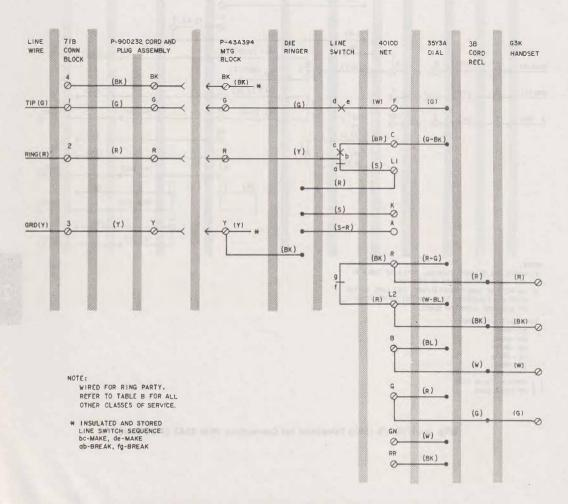
♦Fig. 1—2750A and B Telephone Set, Connections (Current Model)♦
