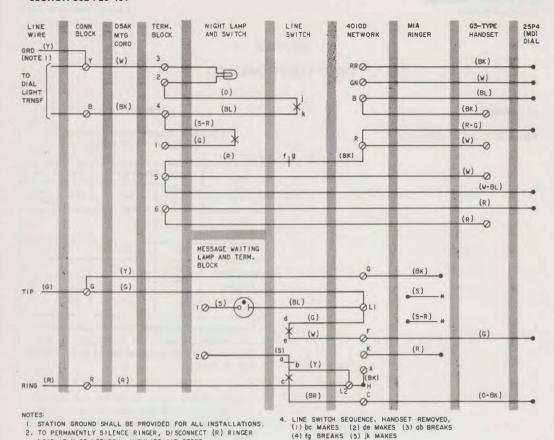
Fig. 1—1702D(MD) Telephone Set Connections With 25P4(MD) Dial, Using D5AK Mounting Cord
