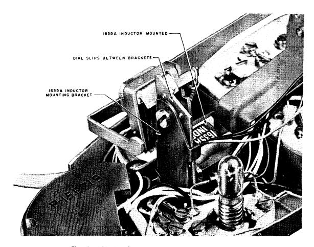
Fig. 7-1635A Inductor Mounted in 701B Telephone Set
