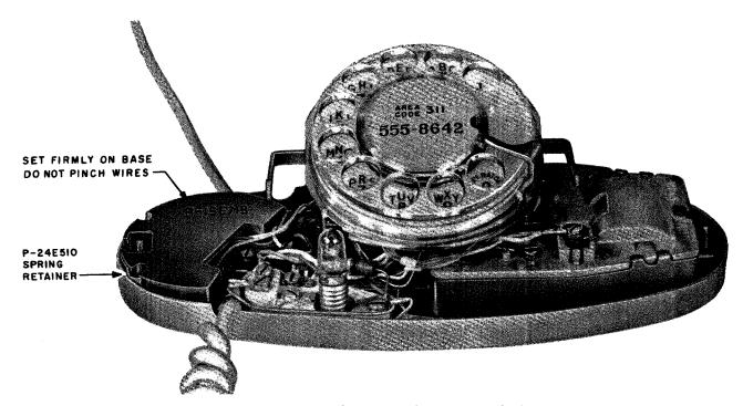
Fig. 10 - P-15E719 Weight Mounted in 701B Telephone Set
