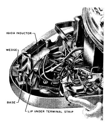
Fig. 5 — Location of 1610A Inductor
