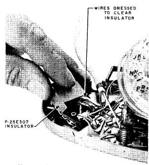
Fig. 8 — Placing Insulator over Terminal
