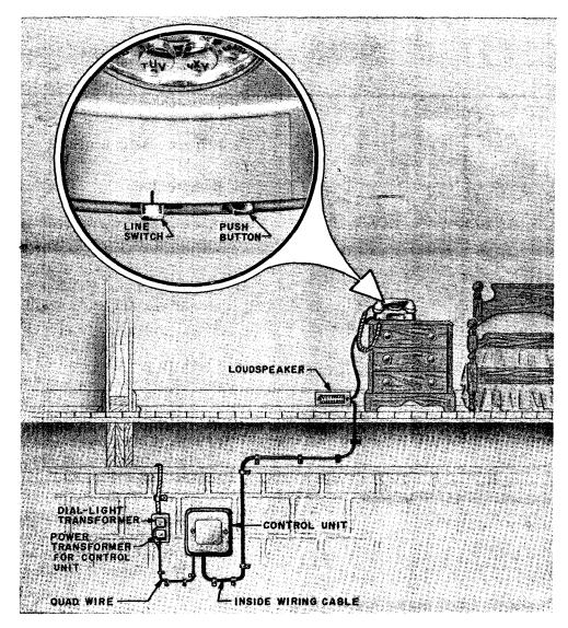
Fig. 3 — Installation of 711B Telephone Set As Used
