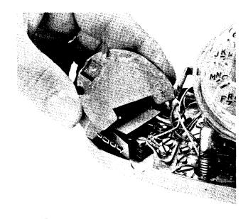
Fig. 9 - Funneling Weight into Position
