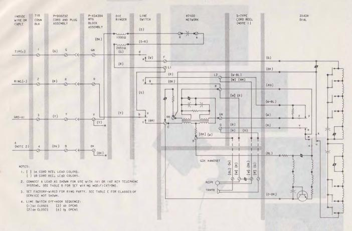
Fig. 4—2750-Type Telephone Set (Later Models)-Connections
