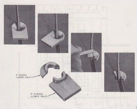
Fig. 3—Removal of Handset Cord Grommet
