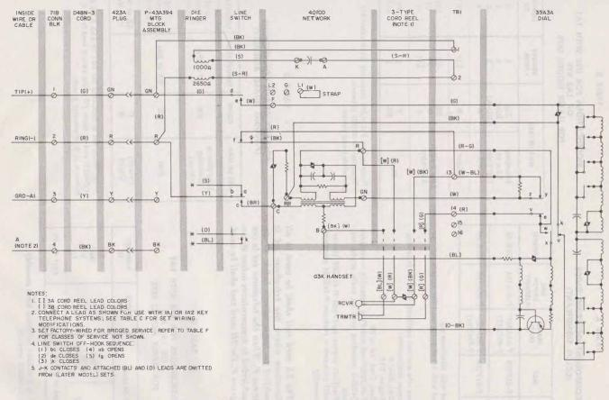
Fig. 5—2750-Type Telephone Set (Early Models)-Connections
