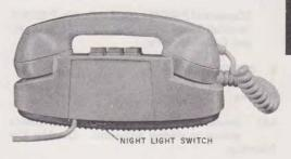
Fig. 2—2702B Telephone Set, Rear—Night Light Switch Location
