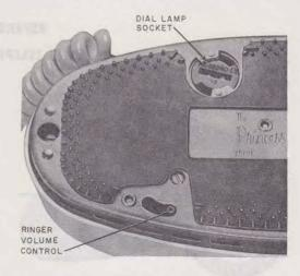
Fig. 3—PRINCESS Telephone Set, Partial Bottom View
