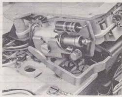
Fig. 5—Polarity Guard Mounted in PRINCESS Telephone
