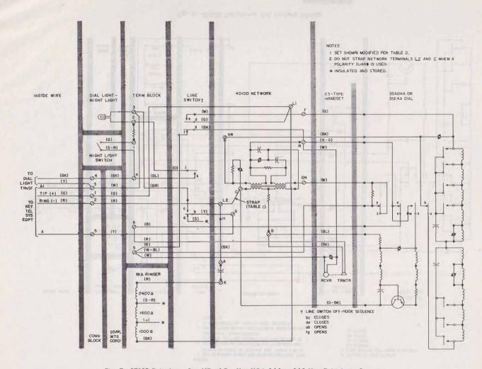
Fig. 7—2702B Telephone Set, Wired For Use With 1A1 or 1A2 Key Telephone System
