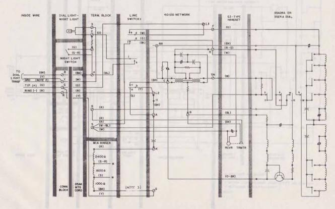
Fig. 6—2702B Telephone Set, Factory Wiring
