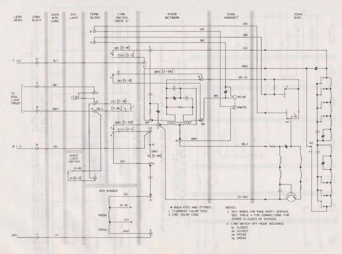
Fig. 4—1702B Telephone Set (Early Production) Using 25H4 Dial and 4010B Network
