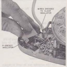
Fig. 8—Placing Insulator Over Terminal
