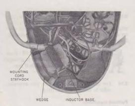
Fig. 5-Location of 1610A Inductor
