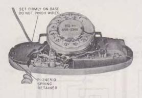
Fig. 9—Location of P-24E510 Spring Retainer and P-15E719 Weight
