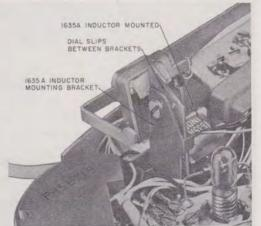
Fig. 7—1635A Inductor Mounted in 701B Telephone Set
