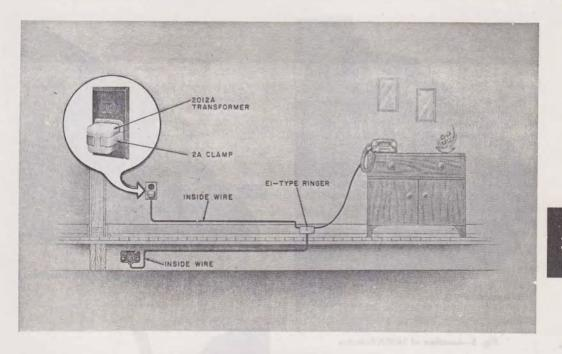
Fig. 4—Typical Installation of 701B Telephone Set
