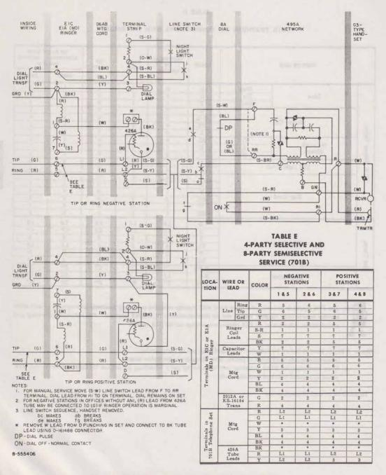
Fig. 15-701B Telephone Set With 426A Cold-Cathode Tube
