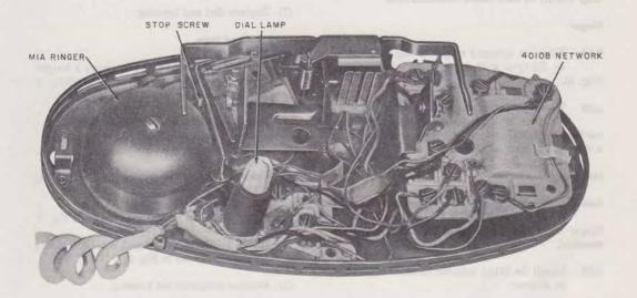
Fig. 3—702-Type Telephone Set, Dial and Housing Removed
