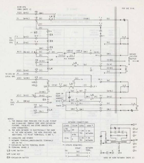
Fig. 2-2660A3 and 2660A4 Telephone Set, Connections
