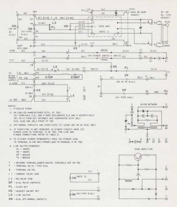
Fig. 2-663A1 Telephone Set, Connections
