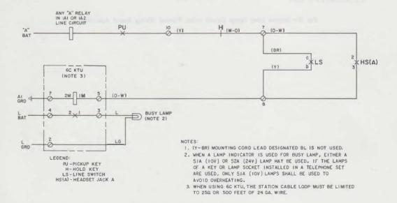
Fig. 5—Busy Lamp Control Circuit Using 6C KTU
