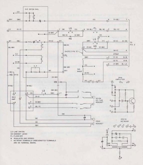
Fig. 1—2636- and 2637-Type Telephone Sets, Connections
