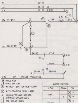
Fig. 4—Station Busy Lamp Circuit With Speakerphone
