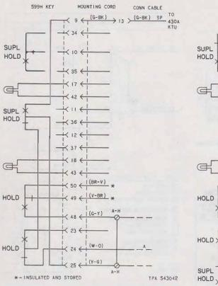
Fig. 6-Priority Hold, Using 599H (MD) Key
