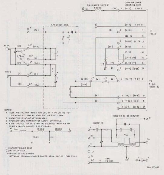
Fig. 1—2630D and 2631D Telephone Set, Connections
