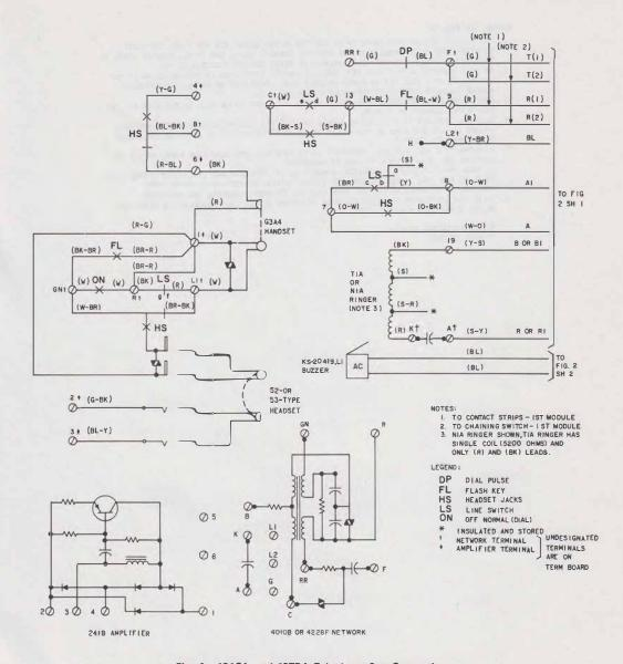
Fig. 1—636CA and 637DA Telephone Set, Connections
