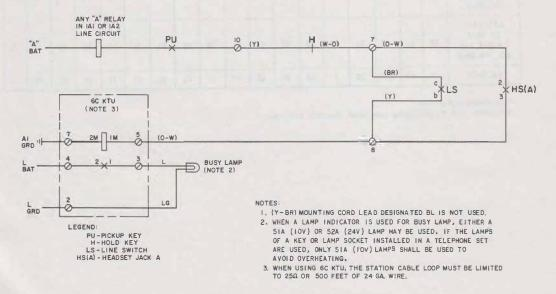
Fig. 5-Busy Lamp Control Circuit With 6C KTU
