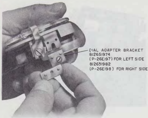
Fig. 14—Placing Dial Adapter Brackets on Rotary Dial When Converting from TOUCH-TONE Dial
