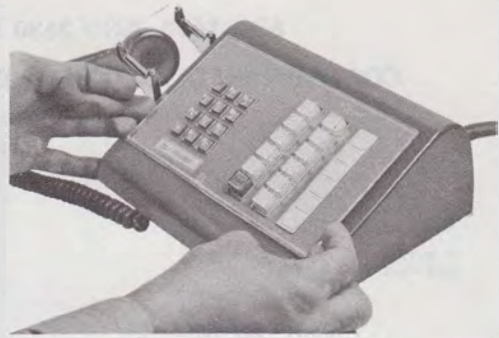
Fig. 2—Prying Faceplate From Lower Bezel of Current Production Telephone Set
