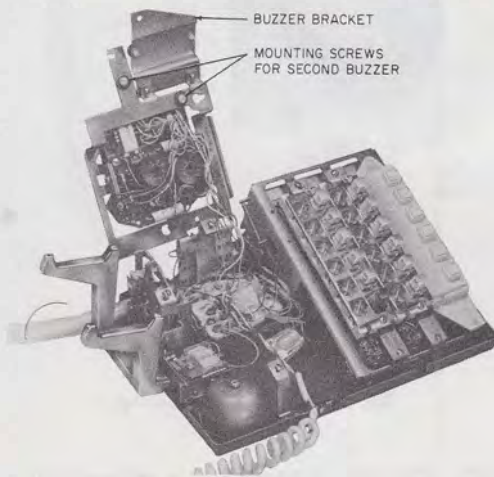
Fig. 17—Mounting Location For Second KS-8109L1 Buzzer
