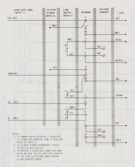
Fig. 1—₱2500M (MD) Telephone Set, Connections♥
