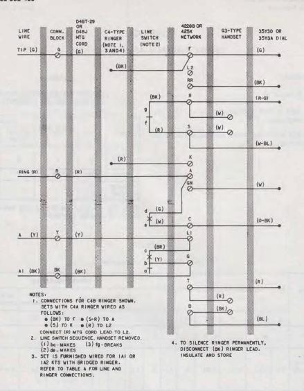
Fig. 1—♦2500M Telephone Set, Connections♦
