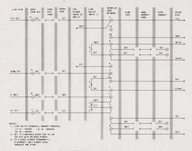
Fig. 2-\$2500MM Telephone Set, Connections
