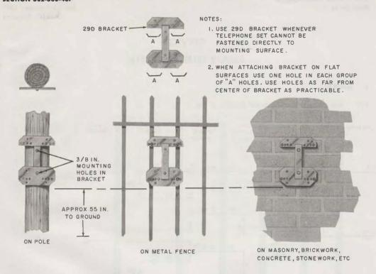
Fig. 2—29D Bracket Mounted on Various Surfaces
