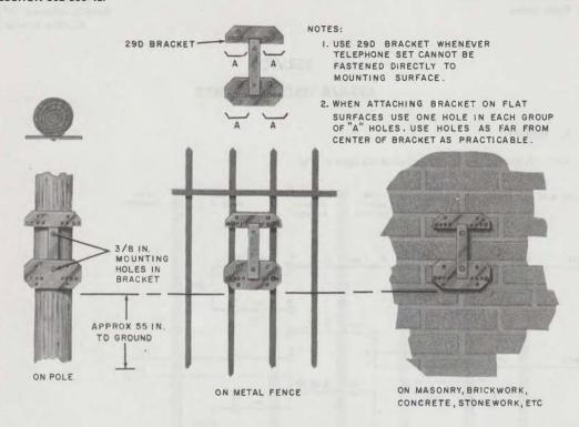
Fig. 2—29D Bracket Mounted on Various Surfaces
