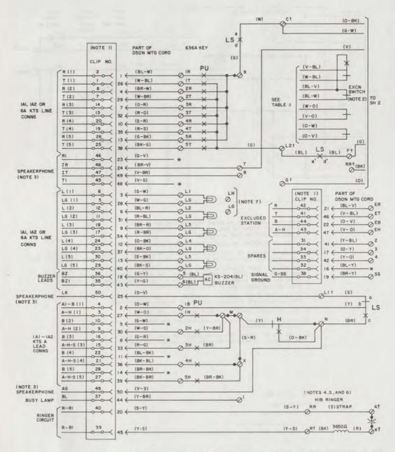
Fig. 2-\$2565HKMS Telephone Set, Connections (Sheet 1 of 2) €
