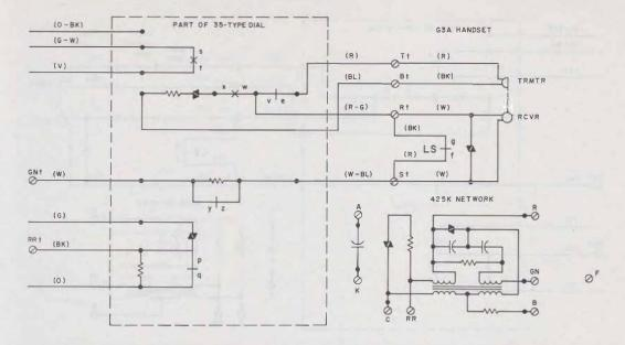
Fig. 1—\$2565HK or 2565HKM Telephone Set, Factory-Wired for 1A1 or 1A2 KTS and Speakerphone Connections (Sheet 2 of 3)\$
