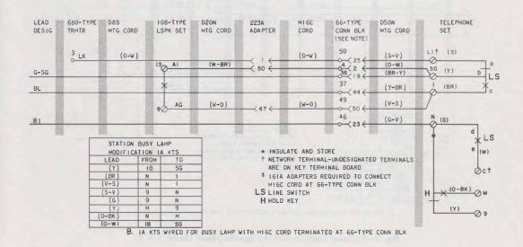
Fig. 3—Optional Features with 4A Speakerphone (Sheet 2 of 3)
