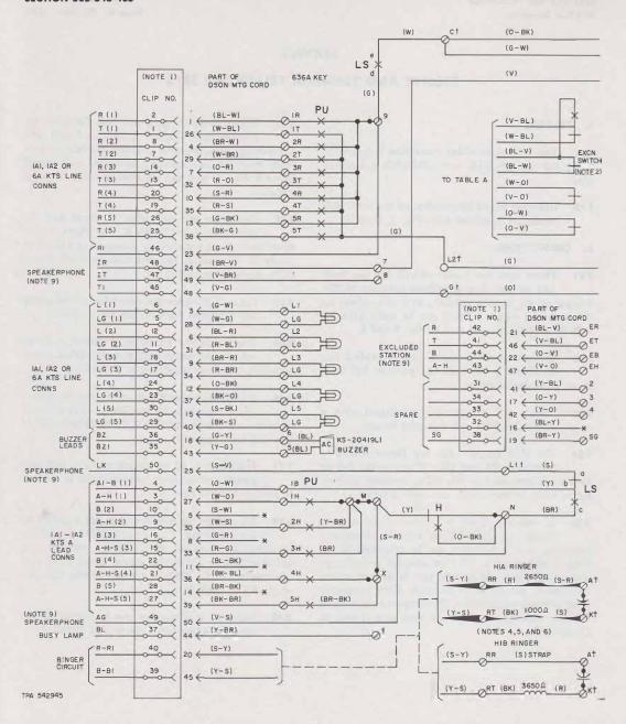
Fig. 1—♦2565HK or 2565HKM Telephone Set, Factory-Wired for 1A1 or 1A2 KTS and Speakerphone, Connections (Sheet 1 of 3)♠
