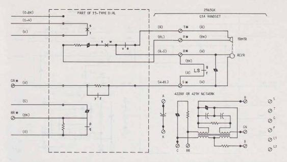
Fig. 1—♦2565GK or 2565GKM Telephone Set, Factory-Wired for 1A1 or 1A2 KTS and Speakerphone Connections (Sheet 2 of 3)♦
