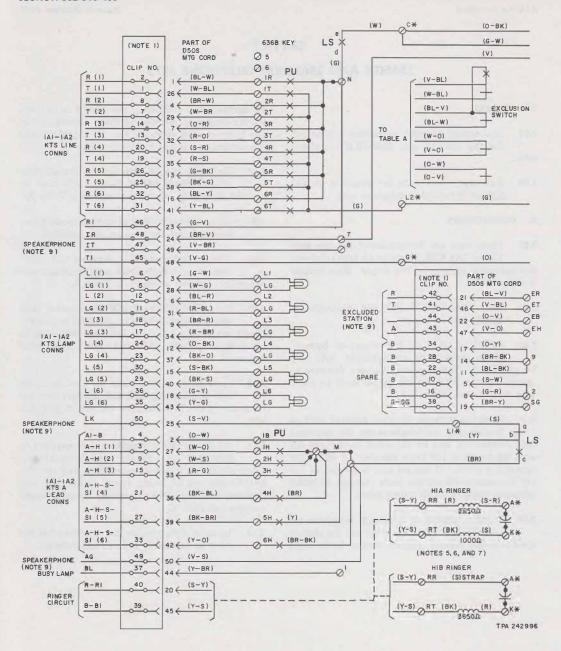
Fig. 1—♦2565GK or 2565GKM Telephone Set, Factory-Wired for 1A1 or 1A2 KTS and Speakerphone Connections (Sheet 1 of 3)♦
