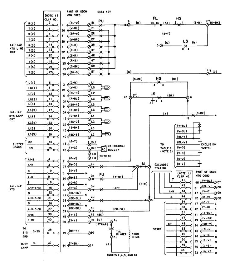
Fig. 5—2563HBM Telephone Set, Connections (Sheet 1 of 2)
