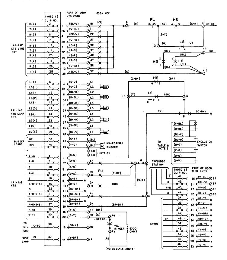
Fig. 6—₱2563HBMS Telephone Set, Connections (Sheet 1 of 2)◀
