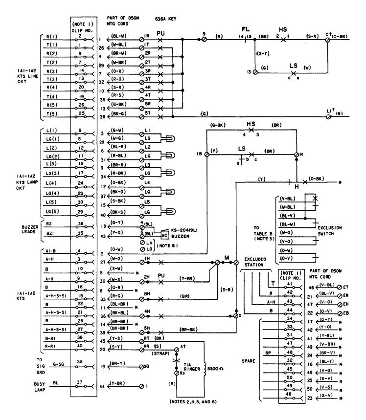
Fig. 4-2563HB (MD) Telephone Set, Connections (Sheet 1 of 2)
