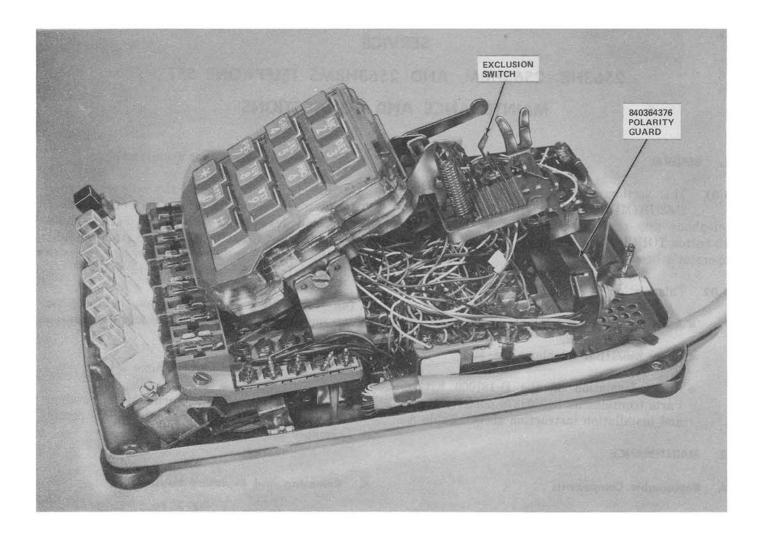
Fig. 1—\$2563HBMS Telephone Set With Polarity Guard Installed€
