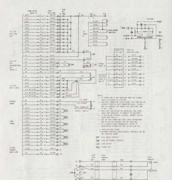
Fig. 2-\$565GKMS Telephone Set, Connections
