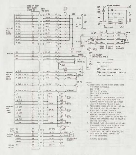
Fig. 4-564HLM (MD) Telephone Set, Connections
