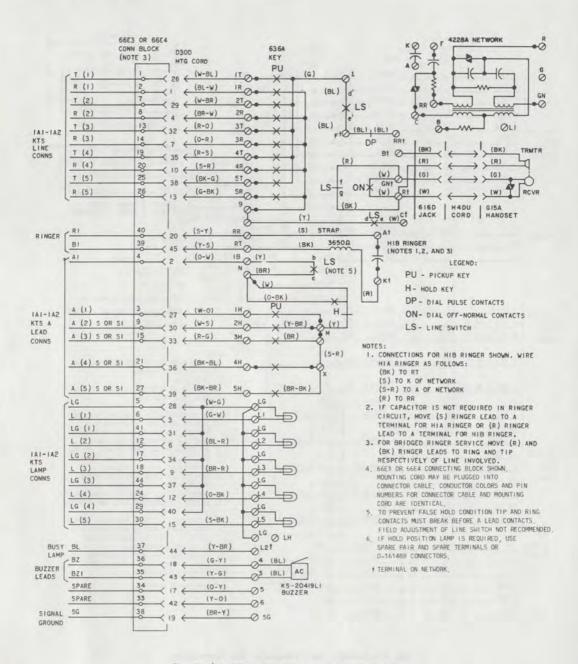
Fig. 5-\$564HLMS Telephone Set, Connections
